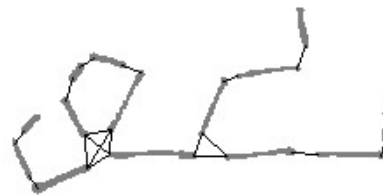
Fig. 11. Link closure “normalizes” data graphs for variations in local link configurations due to relative link lengths.
