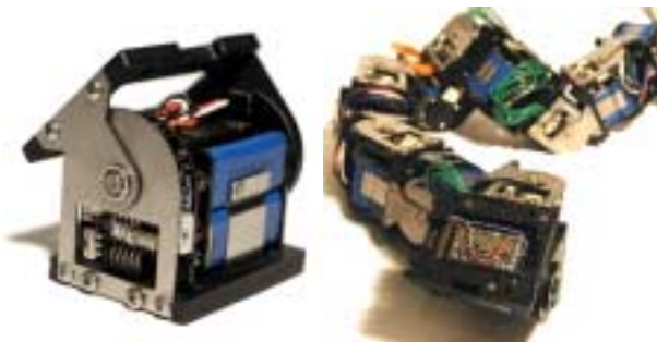
Figure 2. G1v5 PolyBot segment and chain
