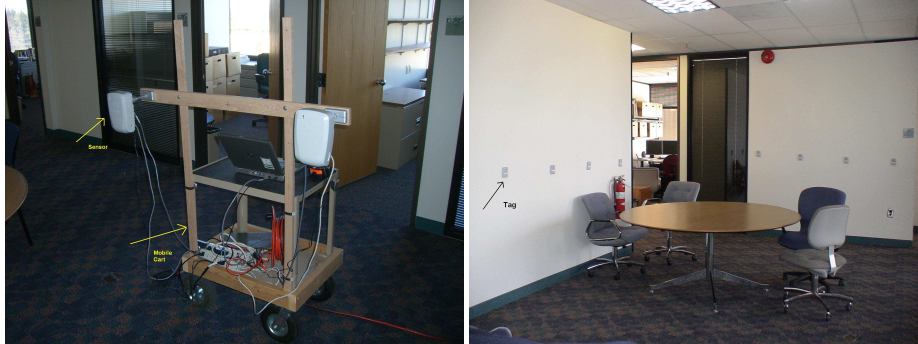
Fig. 7. Left: the mobile cart with two Ubisensors, right: 8 Tags on two walls.
