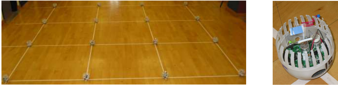
Figure 6: (a) Left panel: node deployment in a 4 \times 4 grid; (b) Right panel: sensor node: Berkeley mote with ultrasonic ranging device.
