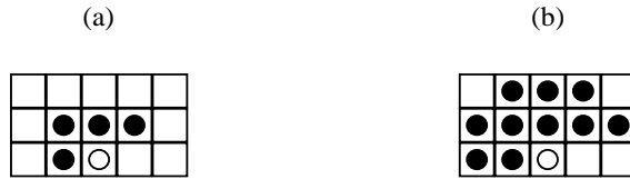
Figure 3. Semicausal pixel neighborhoods of a type suitable for use in the proposed system.
