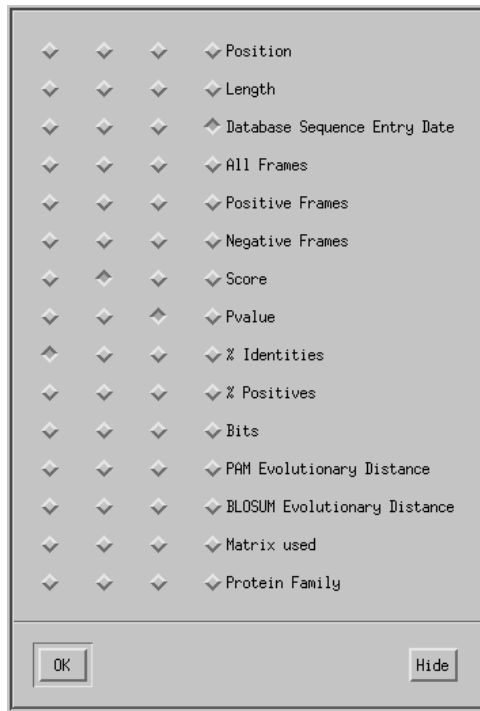
Figure 5: Choosing the axis mapping using the axis mapping panel. The four columns of radio buttons indicate which variables are mapped to the X, Y, Z, and time axes, respectively.
