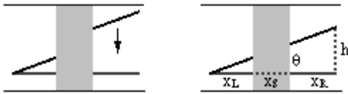
Figure 7: Example of seam width calibration. After the user fits the line on the right side, the seam width x_s can be computed as x_s = (h / \tan \theta) - (x_L + x_R)
