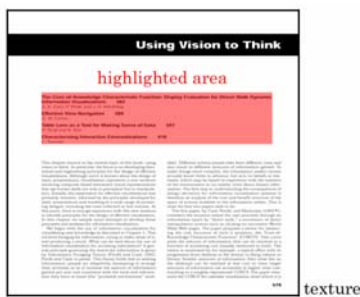
Figure 4: Texture pixels within a highlighted area are blended with a red color.
